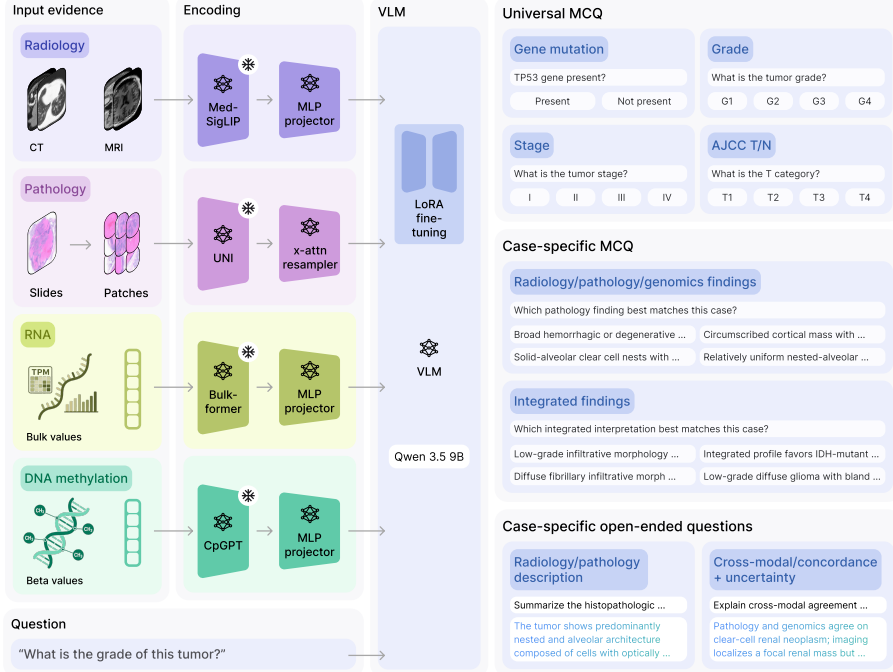
Figure 3: Overview of the proposed multimodal architecture (OncoVLM). Modality-specific encoders map radiology, pathology, and genomic inputs into a shared representation space, which is processed by a LoRA-tuned vision-language model to perform classification and multimodal tasks.
